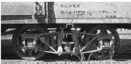
Above: Archbar trucks are still very much in evidence although they are not used much in regular service now. They were banned in interchange service in North America in 1940.
