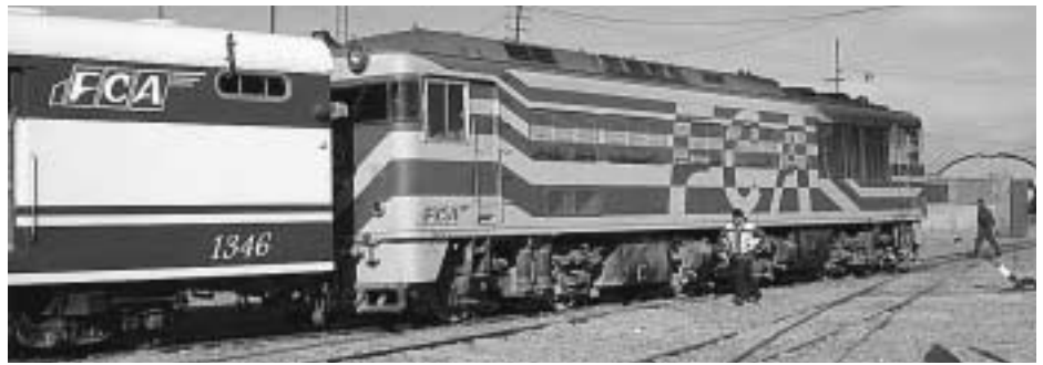
Andina railway locomotive at the head of the special train at Viacha, Bolivia. This locomotive was built by Mitsubishi and has three trucks to distribute the weight.
