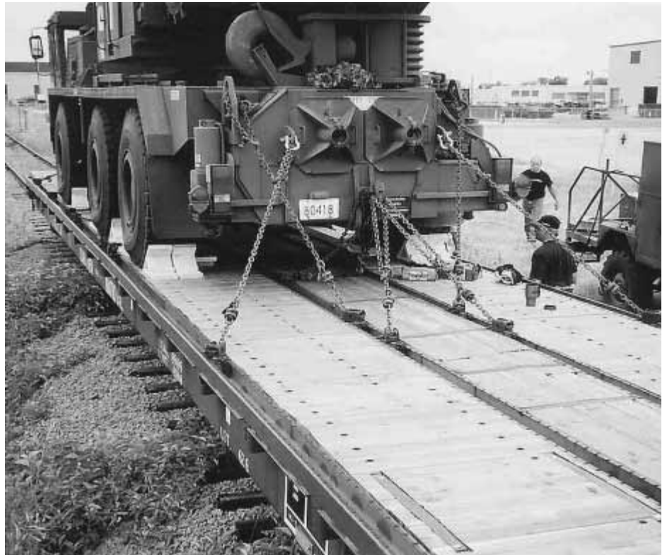
Plunging rear view of crane and flat car. Additional chain tie down channels quite visible.
