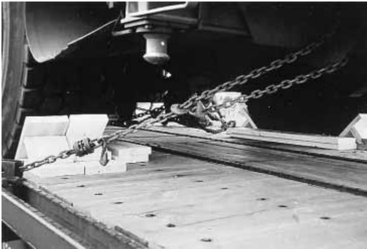
Note the decking and the additional chain tie down running on the outside of the car. The bridge plates used to load the wrecker are visible in the foreground.
