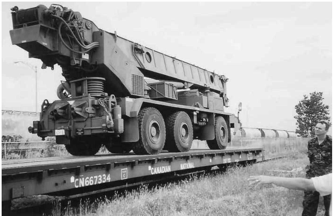
Just driven on the flat car. Show tie down channel welded to stake pockets quite well.
