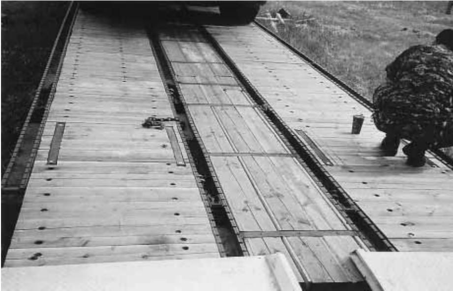
Note the decking and the additional chain tie down running on the outside of the car. The bridge plates used to load the wrecker are visible in the foreground.
