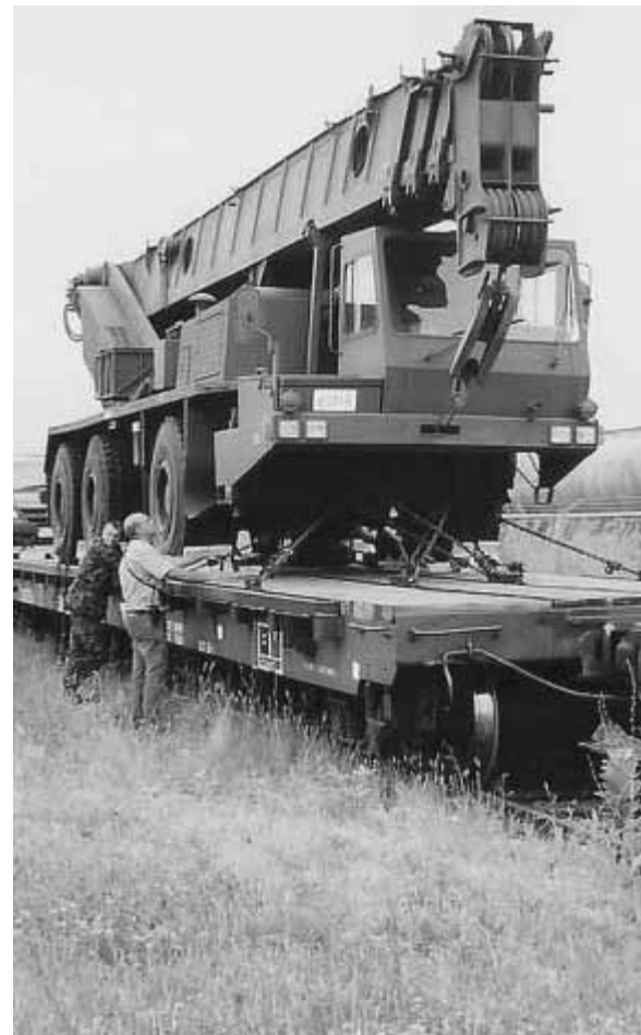
General view of front of crane. Notice end ramp for loading. Note angle of chains.
