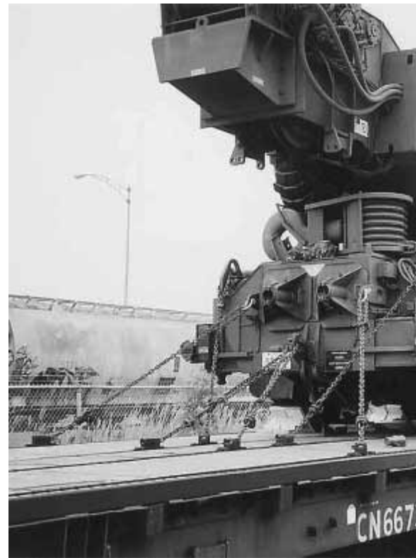
Note the decking and the additional chain tie down running on the outside of the car. The bridge plates used to load the wrecker are visible in the foreground.
