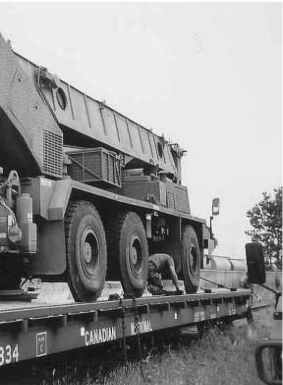
The crane tied down, from the rear. Use of pintle hook for tie down is unusual.
