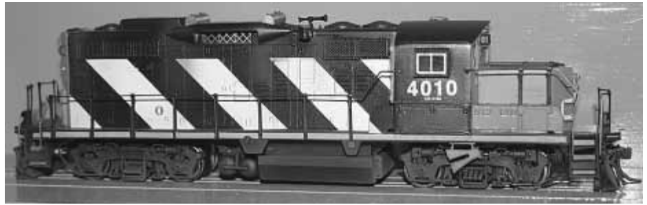
Charls Gendron combined Kaslo shell with Proto 2000 drive to create CN GP9RM.
