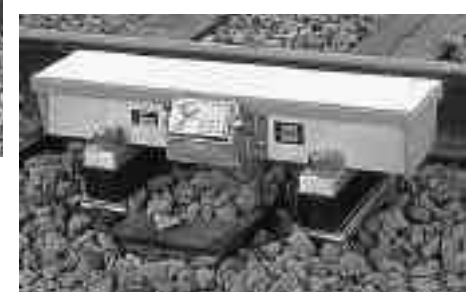
Indusi sensor on lead truck (above) and Indusi magnet on track (right).
