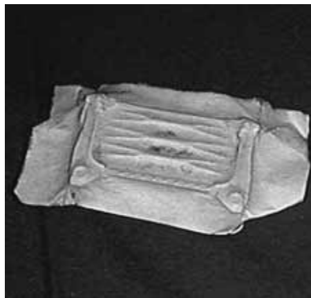
3. A finished moulding, ready to be impregnated with cyanoacrylate — at this point still flimsy..
