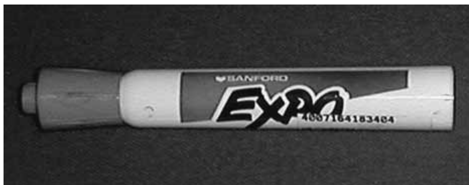
5. Cyanoacrylate that does not soak in does not cure, but forms a scummy film on the surface. A special marker for white boards shows this up. It rubs off where the surface is clean, but soaks into the scum.
