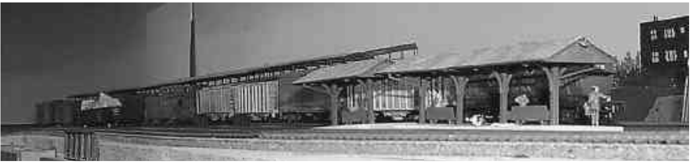
An impressive feature of John's layout is the icing facility at Windsor to handle reefer traffic. Blocks of these cars move through the Detroit tunnel, and must be re-iced before continuing their journey to points east.
