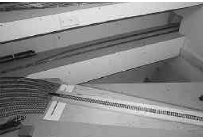
Pivoting plate helps compact staging space requirements. May 2002
