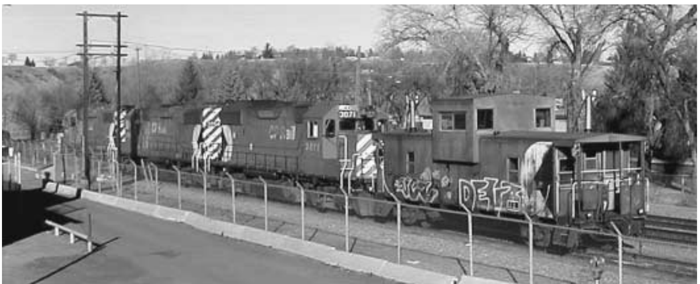
Local turn requires a trio of GP38-2's with dynamic brakes, on account of stiff grades and heavy tonnage.
