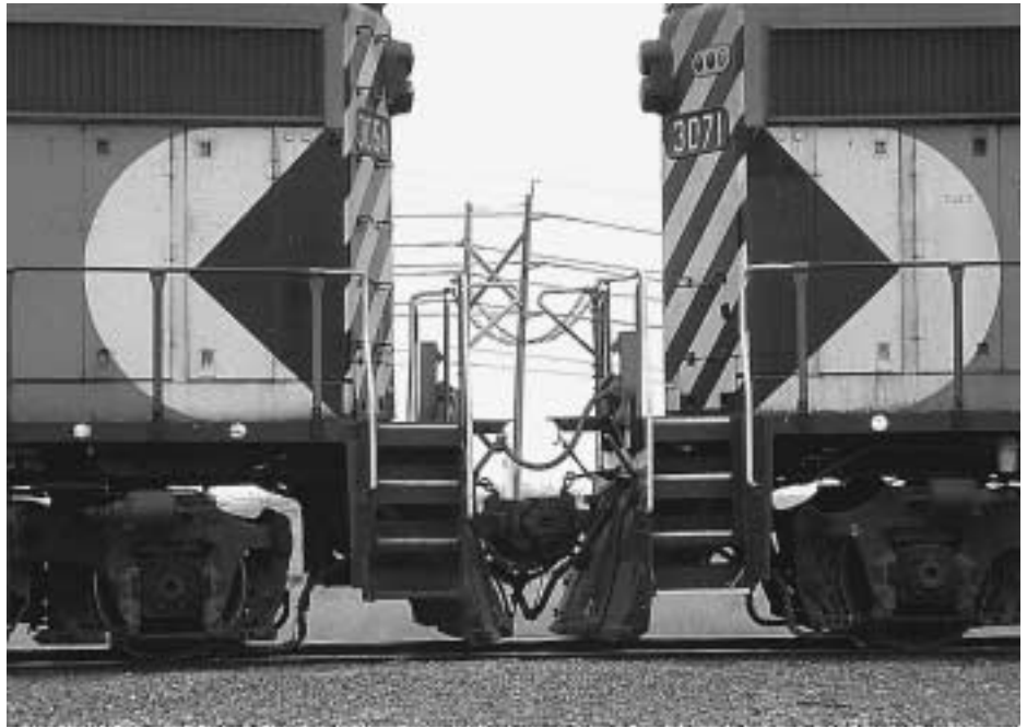
Detail of mu'd GP38-2's. Note railing and safety chains.
