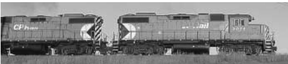
Lead unit of a matched trio of GP38-2's (3107, 3054 & 3071) in Multimark scheme. Notice how the heat from the dynamic brakes has faded the CP Rail lettering.
