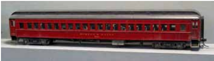
Peter Cunningham: Boston and Maine passenger car #4620 from a Branchline kit of an ex B&O car #800 built by St. Louis Car Company in 1935; purchased by the B&M as part of a program to replace wooden cars in the early 1950s—four-wheel trucks added.
