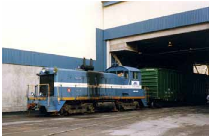
Photo 4: Many pulp and paper mills had company-owned “loks” which were used to perform intra-plant switching. This General Motor SW-900, retired from CN service as #7935, is switching the paper products side of the Howe Sound mill in February 1992. The significance of the sprigs of softwood foliage in the area normally allocated to classification lights is left to the reader’s imagination!
