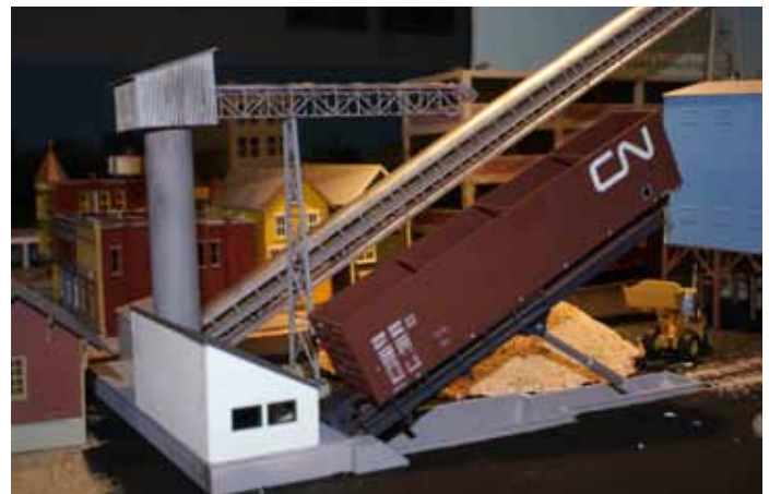
Photo 8: This form of wood chip unloader serves both bottom and end unloading cars. An article describing its construction was included in the November 2009 edition of The Interchange (Issue 439). Walthers conveyor kits were used as “building blocks” for conveyor system models and, in fact, for the transmission of mill fluids. The conveyer elements were used to move the chips from the unloading structure to storage, and from the same unloading structure to the top of the digester. Beyond the chip storage yard is a dock at which recycled paper and rags may be unloaded into the digester building. Also visible is a portion of the lime kiln.
