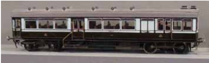
Dave Venables: P4 L&NWR Railmotor by Mallard Models; built from a Mallard etched brass kit; painted with a combinations of spray, brush, and lining pencil; built to P4 standards, which are basically 4mm to the foot and 18.83mm track gauge.
