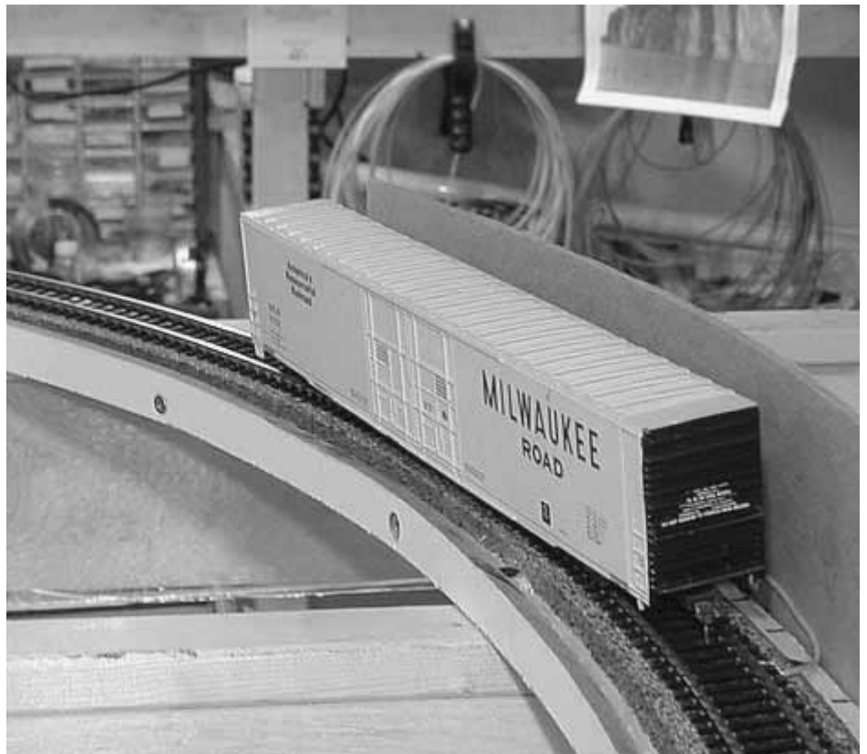
View from inside the curve with outside flange put in place. Testing clearances with the 89 footer showed that I needed more inside clearance, hence the strip of hardboard screwed to the inside of the roadbed. There will be a Plexiglas inside fence reaching up to diesel walkway level to prevent derailed cars from falling to the floor.
