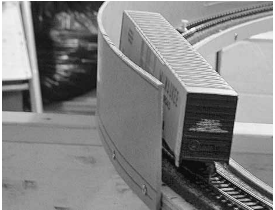
The vertical flange made of \frac{1}{8} " hardboard follows the 29 inch outside radius horizontal curve of roadbed very easily, but is otherwise extremely stiff in the vertical plane. Our trusty 89 foot hicube is checking clearances. The track is super elevated, hence the lean on the hicube boxcar.
