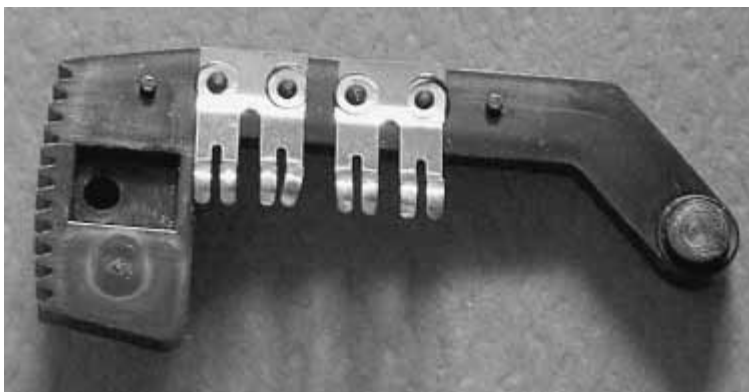
Figure 3: Lever and sliding contacts.
