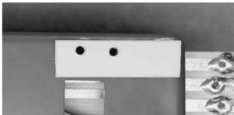
Figure 6: Mounting pads and drilled holes for micro-switch.
