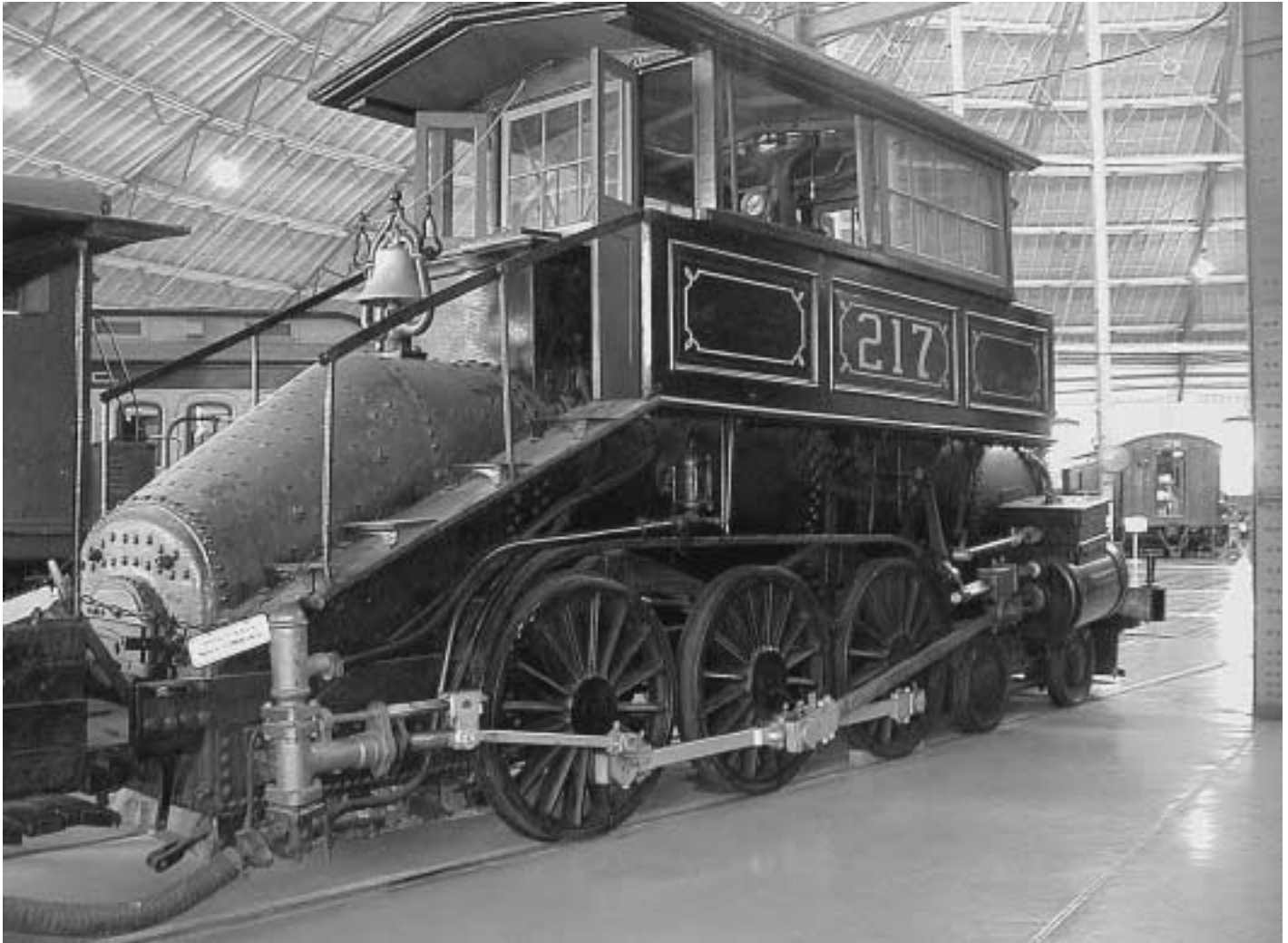
Rear view of "cab-over-engine" design (Mother Hubbard) Ten Wheeler. An eccentric on the rear axle drives the water injector pump.
