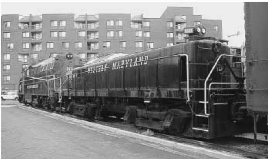
Western Maryland BL2, in “Speed ball” scheme, with a slug rebuilt from and ALCO switcher. The stainless steel hump belongs to a B&O RDC2 on the next track.
