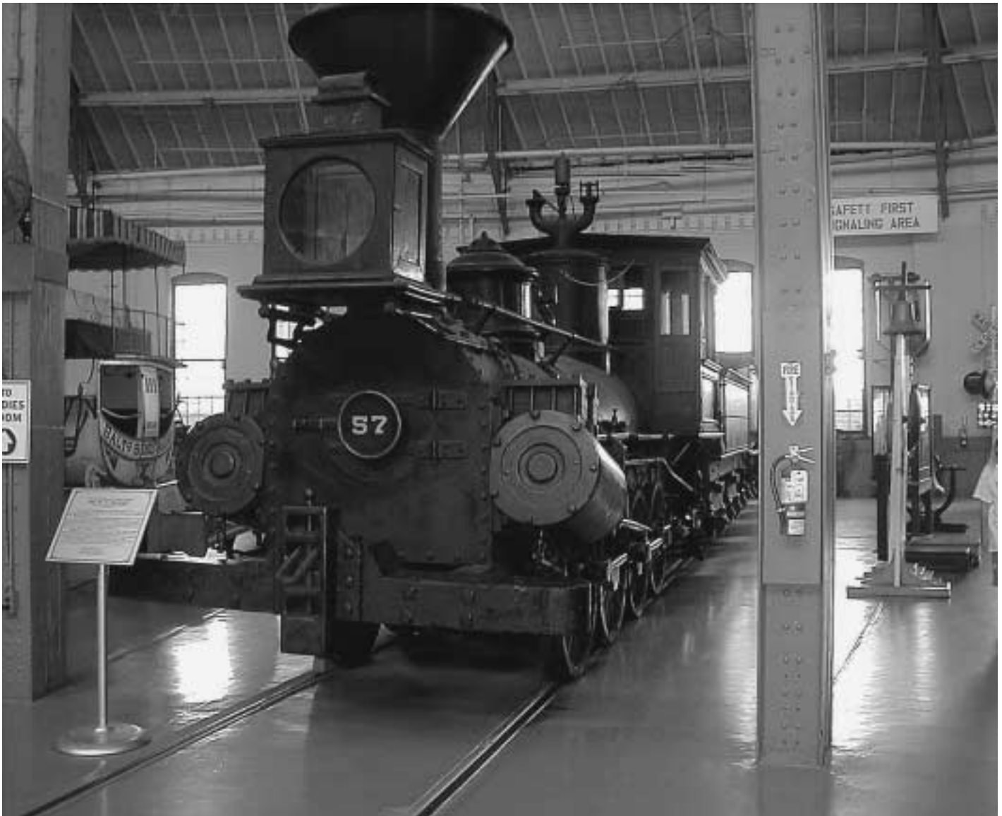
0-8-0 heavy freight locomotive. Note the absence of "Cowcatcher" pilot, the link & pin couplers and the size of the kerosene lamp.
