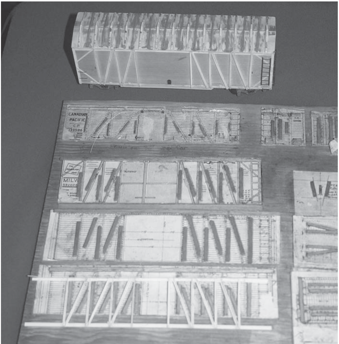
Plans form basis for jigs created from balsa strips, and are even more useful when constructing multiple cars.
